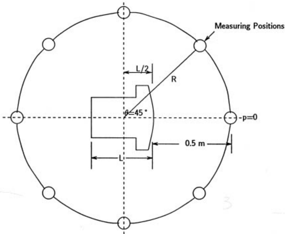
**Figure 3—Position of VDT for magnetic field testing (top view)**
