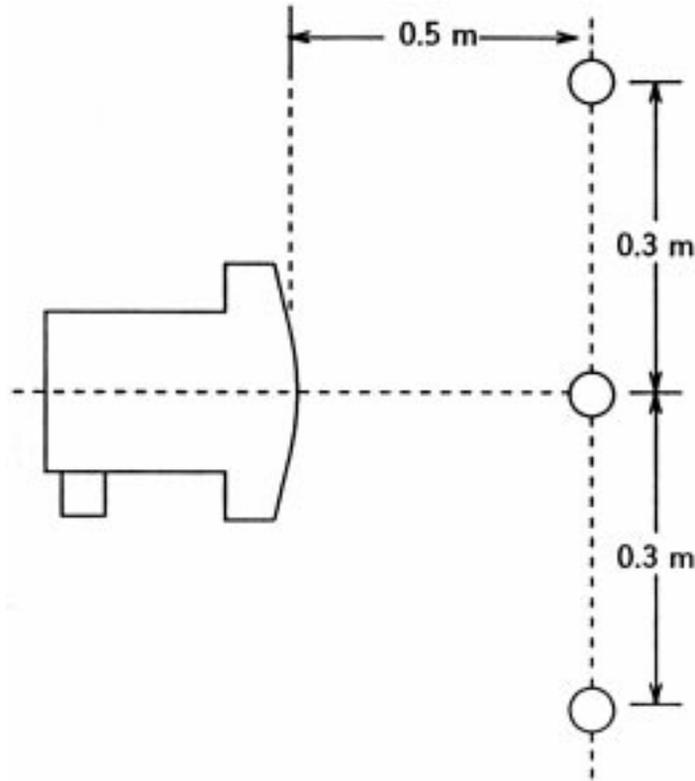
**Figure 4—Position of VDT for magnetic field testing (side view)**
