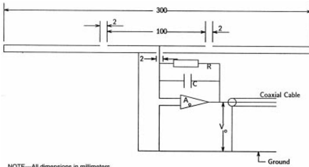
Figure A3—Simplified electric field meter probe and detector circuit
