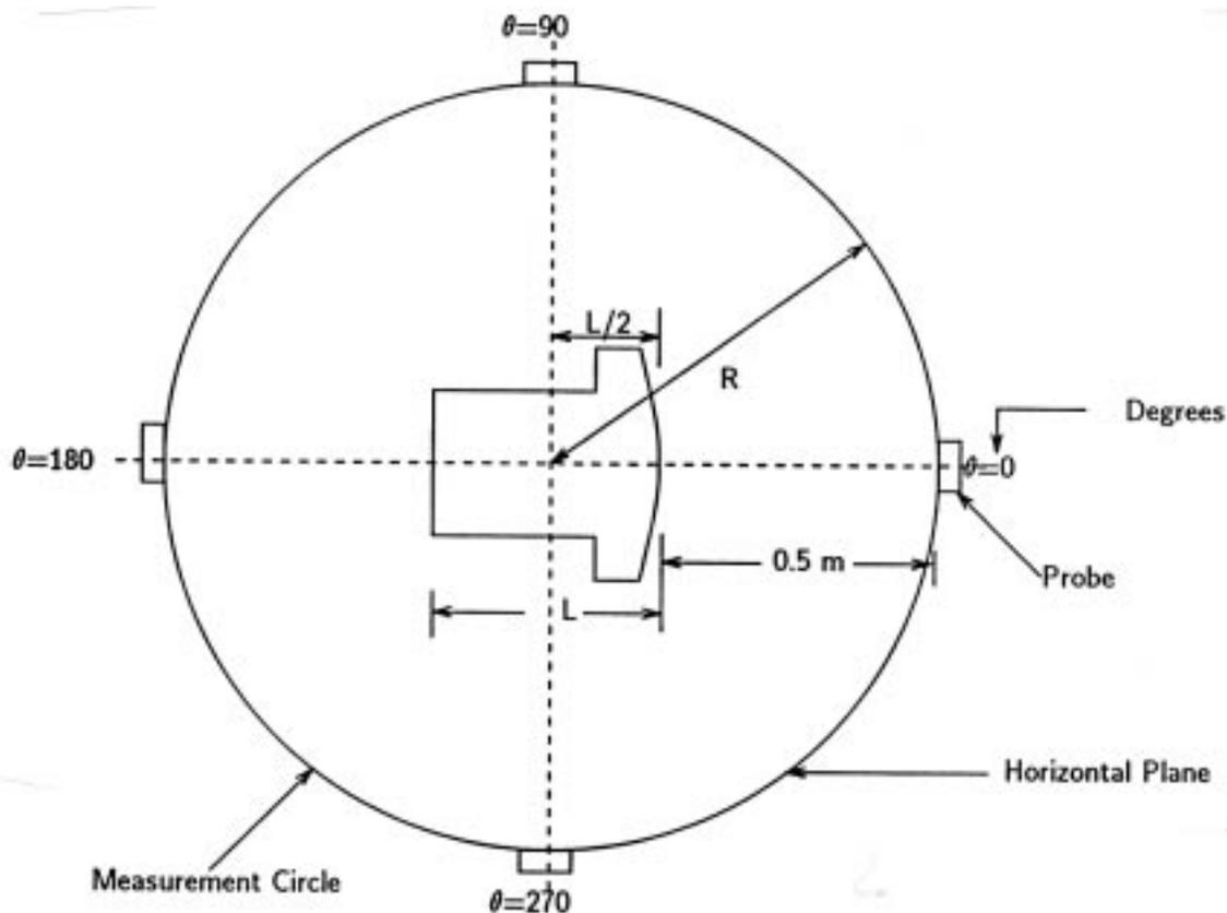
**Figure 2—Position of VDT for electric field testing (top view)**
