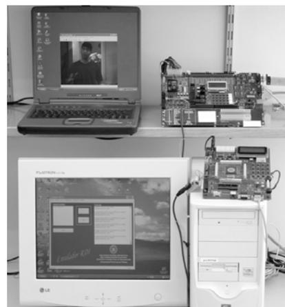
Fig. 7 Testbench of the DAB/DMB receiver
