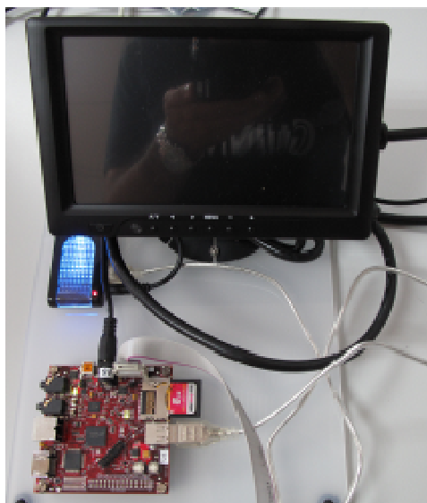
Fig. 3. Tarjeta Beagle Board
